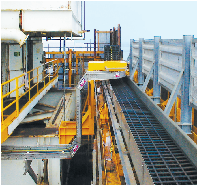
E4 e-chain® with several extension links for extreme fill weights, guided in igus® steel trough over long travel distances in rough seas
