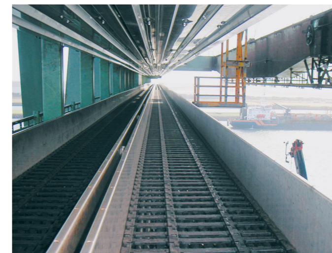
igus® system E4 with extension link on a ship loader for coal handling. Travel 105m, speed 240m/min, fill weight 53kg/m
